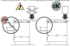
For all models shown, the assembly must be completed with the workstation system assembly guides.
